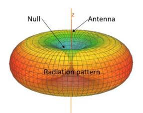
Transmit or Receive, λ/2 and smaller, antennas have almost exactly the same aperture, pattern & gain
