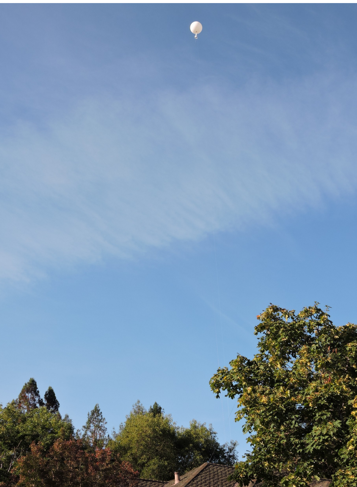
Balloon supported 2m halo at 160' AGL, connected to ground-mounted transceiver by AWG @28 SWTL
