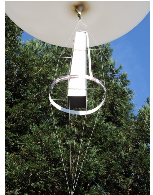
Balloon supported 2m halo at 160' AGL, connected to ground-mounted transceiver by AWG @28 SWTL
