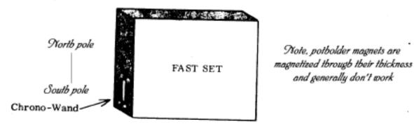
Now move the Chrono-Wand to the same spot on the bottom of the right side of the clock. If you hold the magnet in this position the pattern will advance one every second.
