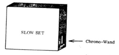
To set the clock, advance the time using the "fast set switch" through a full twelve hours, then continue until you're within an hour of the correct time. Then move the Chrono-Wand to the "slow set switch" advancing the time to the correct minute. If you advance the time too far repeate the process. (See footnote 14 for accurate setting)
