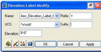
After an Elevation Label has been placed, you can regain access to the main dialog by using the Context menu (ElevationLabelModify) - see illustration left. Because the Attribute Text is embedded within these MvBlocks, using the Elevation Label Modify dialog is the easiest solution for changing the text labels.
