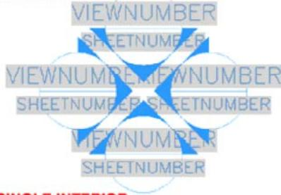
In Architectural Desktop there are two primary Elevation Callout Types: **Elevation Single** and **Elevation Four Way**. The Single Elevation Callout Mark is basically one direction of the Four Way Callout Mark so if you can figure out how to use the more complicated one the single one will be easy.
