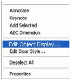
Materials can be assigned to Objects by the Style as illustrated to the right or directly to a specific Object as a Style override. **Select** the specific **object**, **right click** on your mouse to invoke the context menu and select **Edit Object Display...**
