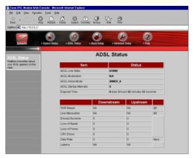
From here, you can verify whether your ADSL connection is active or not (**ADSL Line State Status** will read **SHOWTIME**). You can also monitor related ADSL parameters; for example, how fast the Bridge is transferring data.
