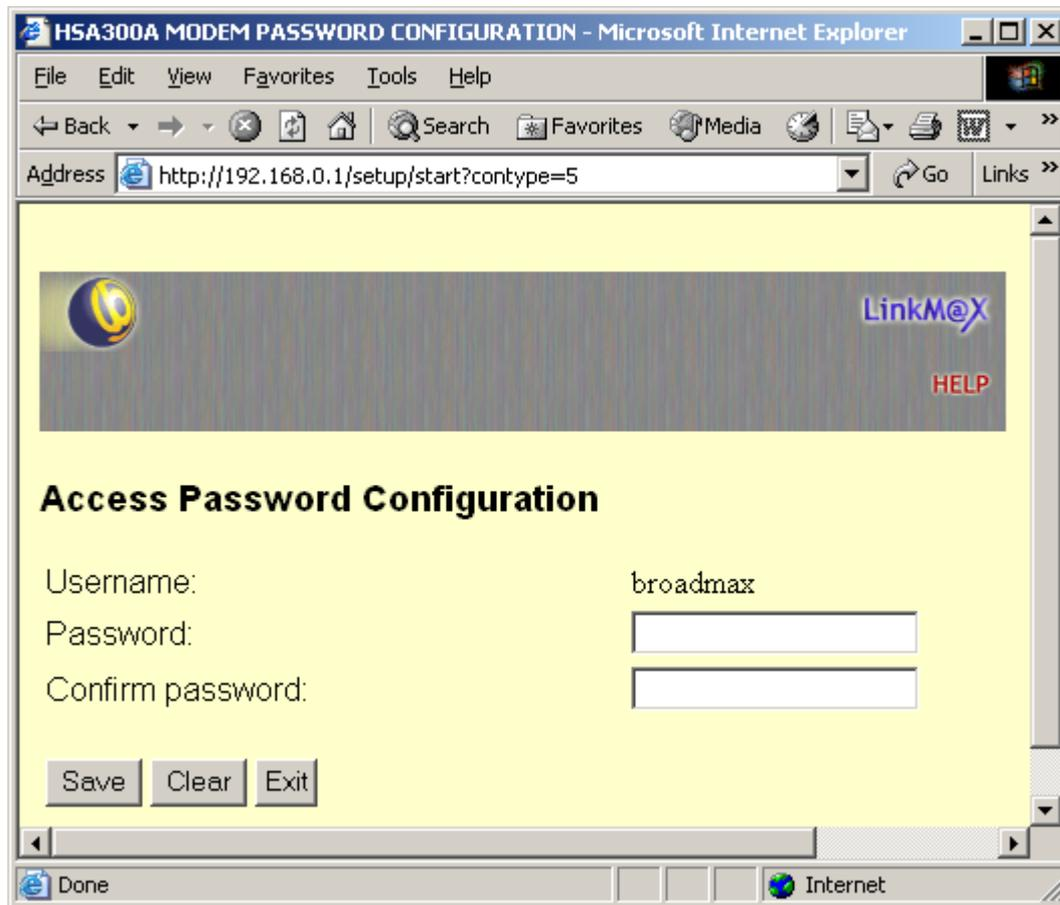
To change Access Password for the web configuration, type new password in the **Password** box and retype it in **Confirm Password** box. Click **Save** to validate change.
