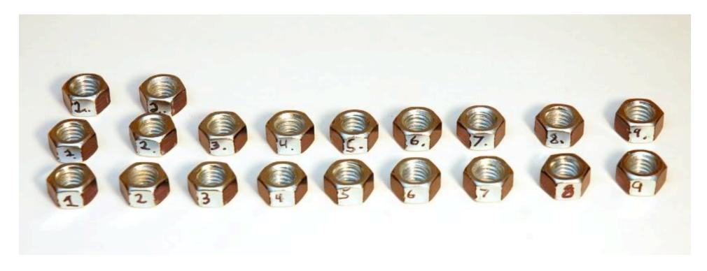
**Notes:** Pictures and data from DavidB's Garage Journal <u>thread</u>. This test was more controlled than the previous one. In this test the wrench was held in a vise between two pieces of wood and a torque wrench was used to torque a nut in the box end to 30 ft-lbs. The nut was colored using a Sharpie marker to better show the contact areas.
