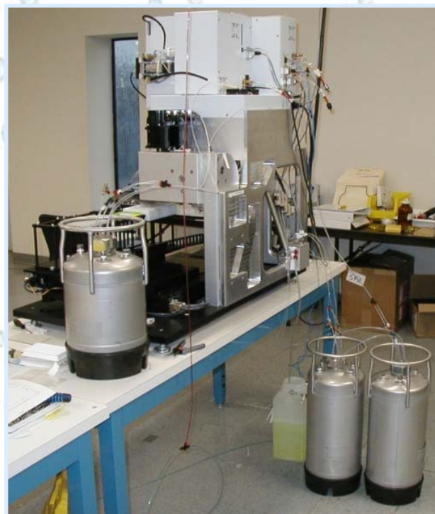
2-Gal and 5-Gal High Pressure Tanks with Screenmaker
