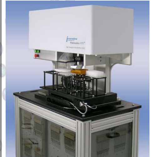
Nanodrop II Dispensing to 1536-Well Plate
