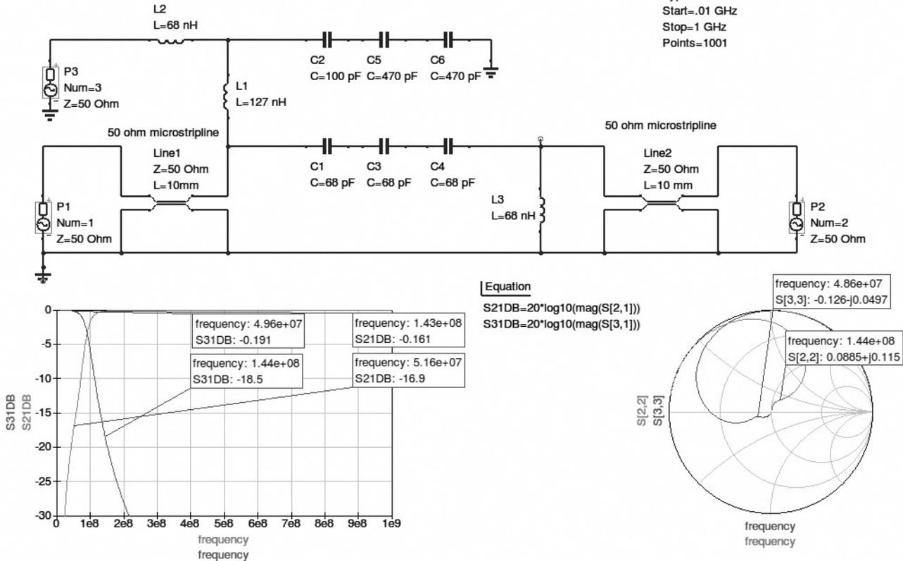
Figure 2: HF/VHF+ diplexer used with the All-Band antenna.
