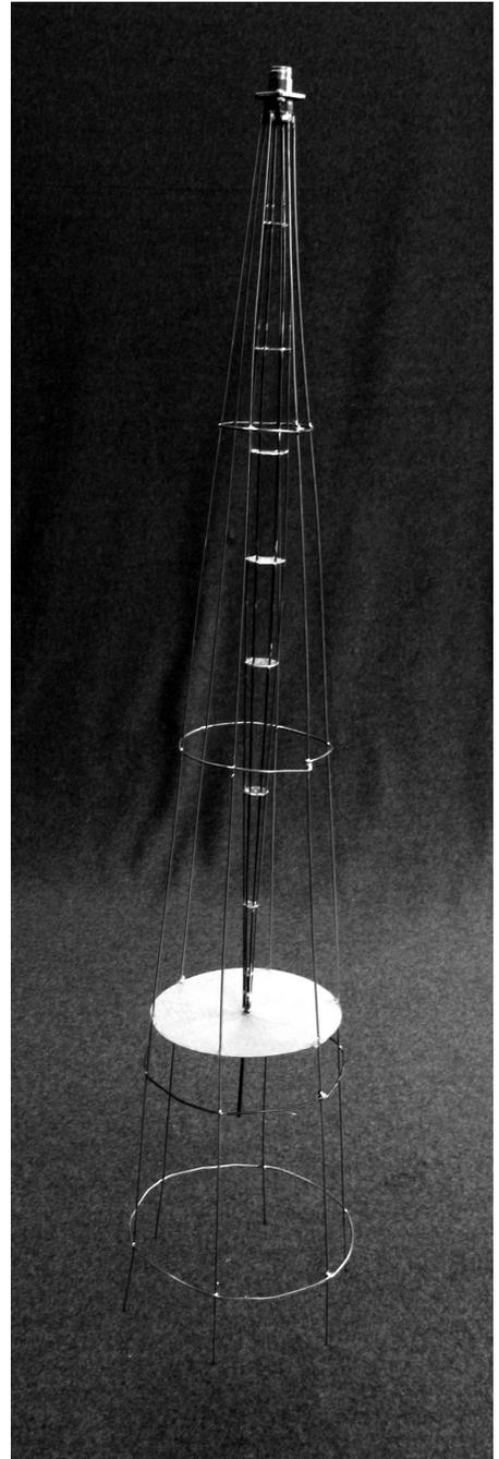
*Photo 1: Detail of coaxial end of the bottom launcher showing an N connector mounted on a copper flange(left) and the complete bottom launcher(right) with both the inner and outer assemblies made from 1/16" brazing rod. A sheet plastic or Styrofoam disc is used to maintain alignment, spacing and shape between the inner and outer conductors. The outer conductor is held in shape by copper wires formed into circles and soldered around the outer rods.*
