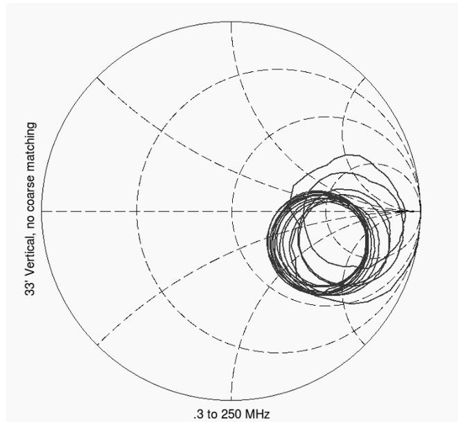
Figure 3: Measured  $S_{11}$  (50 ohm reference) of 33' vertical (without SWTL) with 24" metal disk improving a sod+ground rod image plane. Improvement by this disk is evidenced by the cleaner, lower impedance circles at higher frequencies. Note that in operation the antenna actually uses a transformer to shift the circles' centers to nearer 50 ohms.
