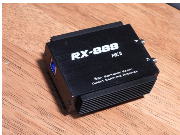
RX888 v2 bottomv view, "RF end" SMA connectors are on the right, USB on the left.
