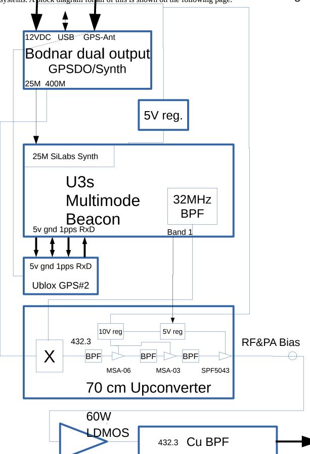
As seen in the block diagram, the entire system is to run from 12-14 VDC with a goal of requiring no more than 15 amperes from the donated power at the site.
