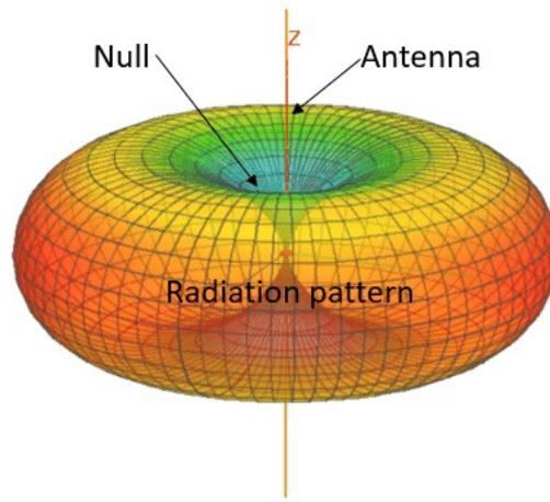
Transmit or Receive,  $\lambda/2$  and smaller, antennas have almost exactly the same aperture, pattern & gain
