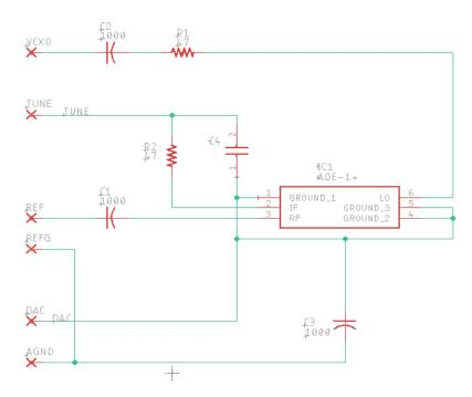
Figure 6: PLL PCB Schematic
