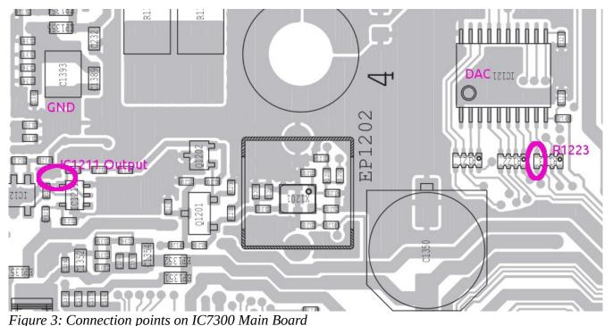
Connections to the radio are made by way of small diameter magnet wire and soldered to the PCB and (carefully) soldered to the SMDs of the radio; resister array R1223 (end resistor) near the DAC and IC1211 and ground (attached at nearby capacitor which is also grounded).
