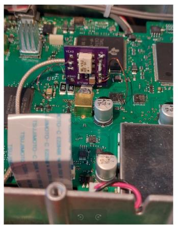
Figure 2: PLL PCB mounts near the center of the IC7300 Main Board on the bottom side of the transceiver. A solder lug is bent at right angles and holds the board securely by way of an existing mounting screw.
