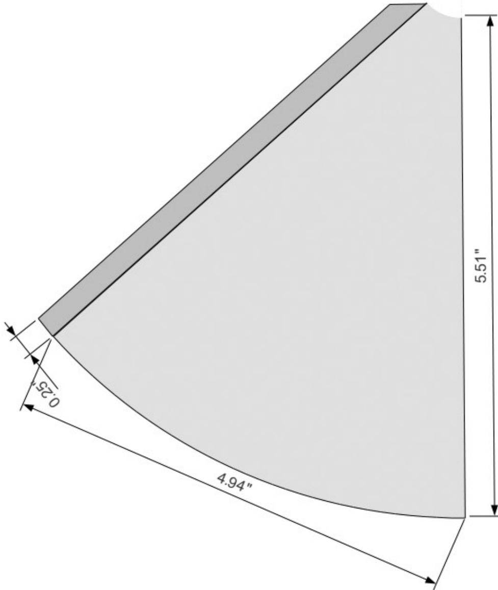
**Figure 5 Template for brass portion of 144 MHz launcher outer cone.**
