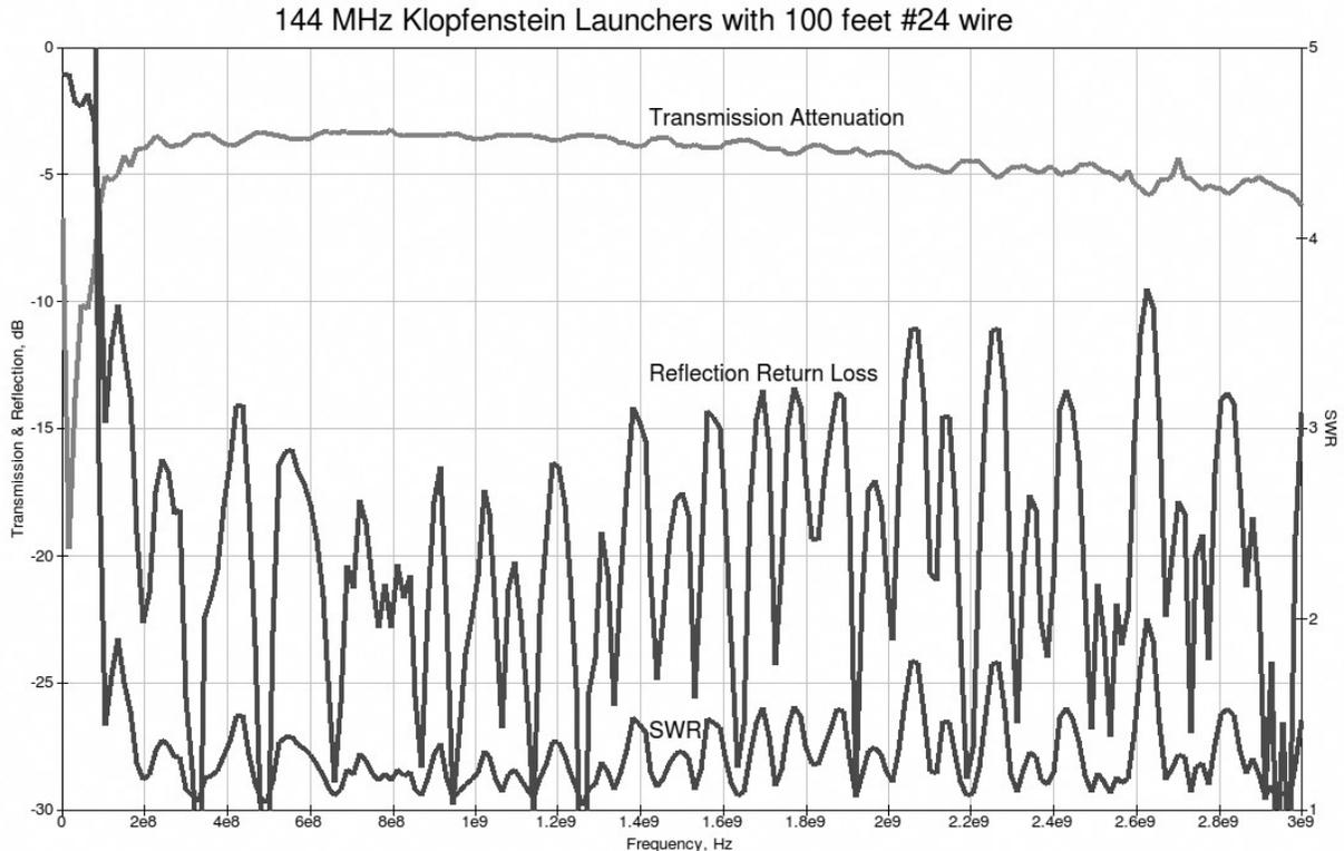
Figure 7: Measured Performance of 100' SWTL line with 144 MHz Launchers
