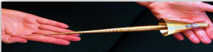
*Klopfenstein taper with SMA connector and brass portion of cone*
