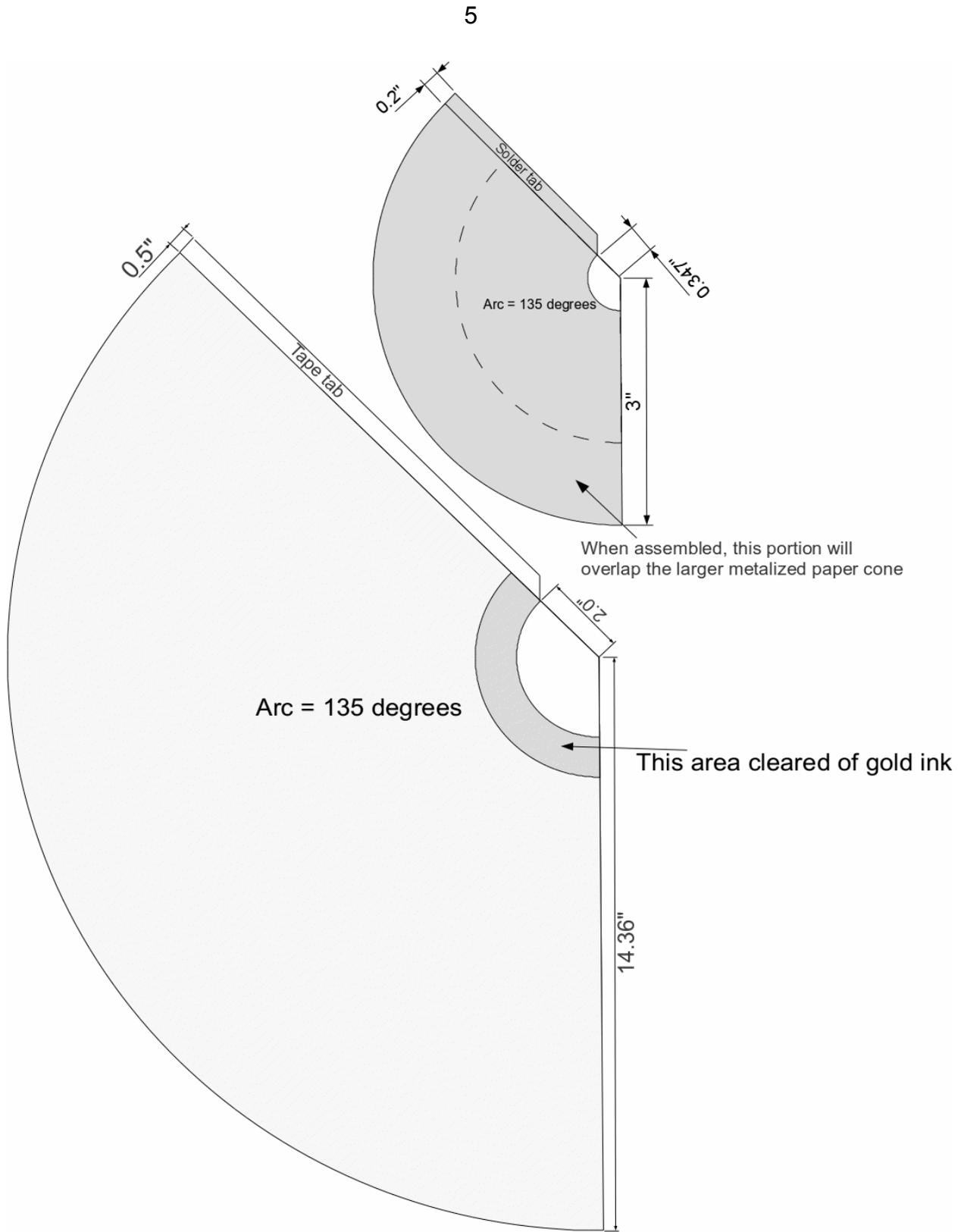
**Figure 2A Cone patterns before folding, metalized paper and brass shim stock**
