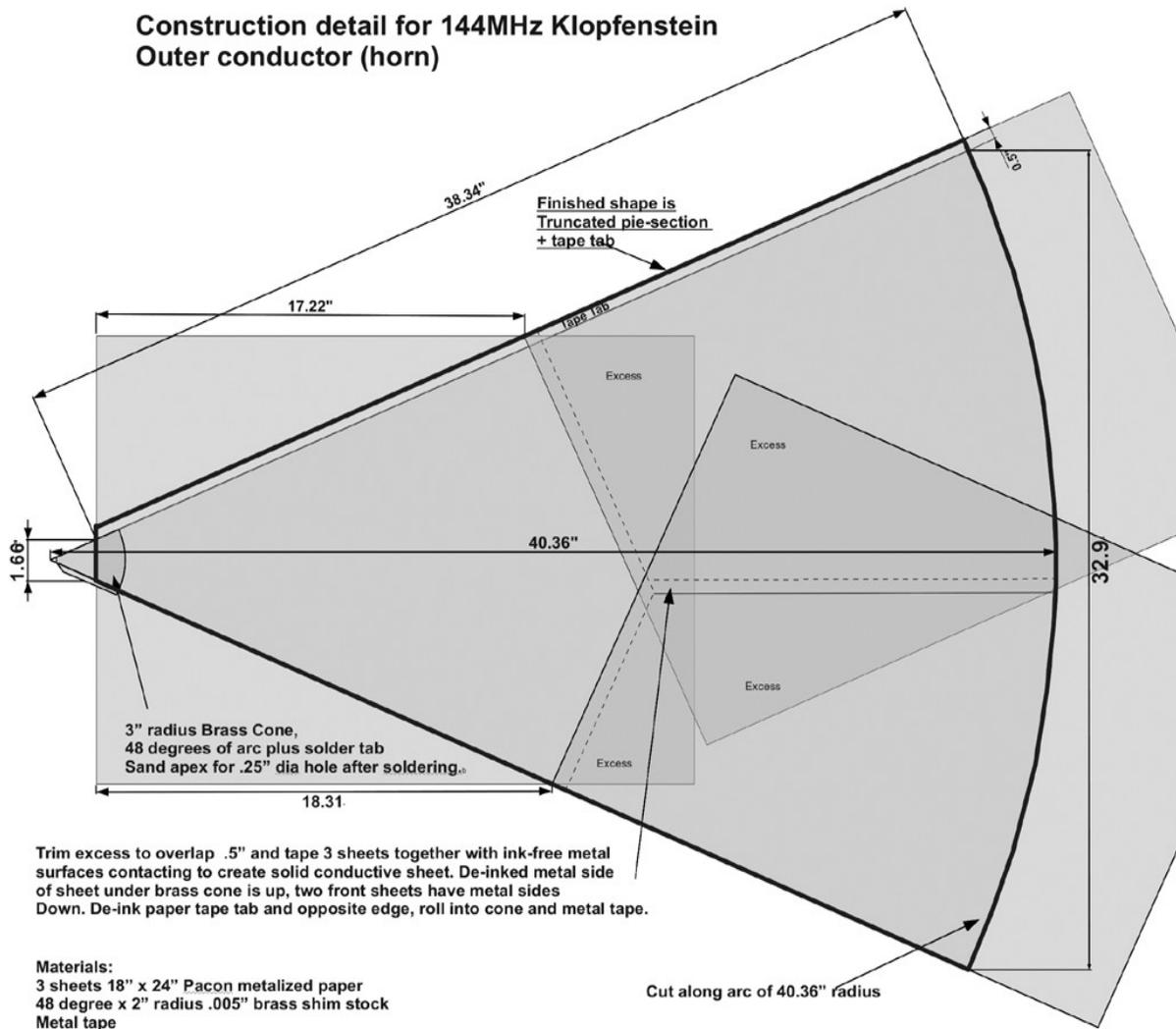
**Figure 4** The paper cone for the 144 MHz version of the launcher requires three 18x24 inch sheets of metalized paper.
