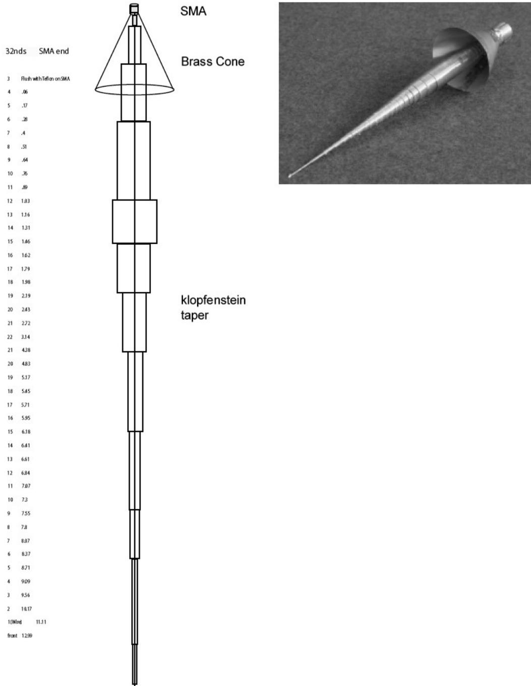
Figure 2B. Dimensions of inner launcher tapered conductor sections made from K&S Metals brass tubing (in 32nds of an inch) vs. position from the SMA connector for the 400 MHz launcher.
