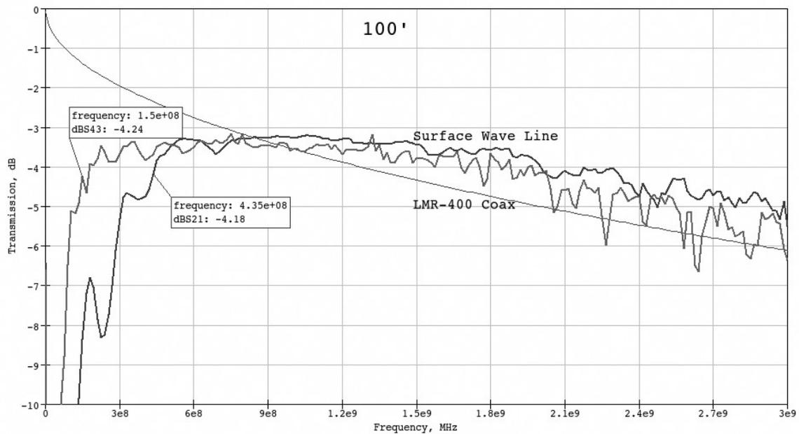
**Figure 1 Measured performance of SWTL compared with measurement of Times Microwave LMR-400 coaxial cable. Plots of 100 feet of #24 AWG conductor with a pair of 400 MHz launchers and a pair of 140 MHz launchers are shown. The main difference between these is the cut-off frequency**
