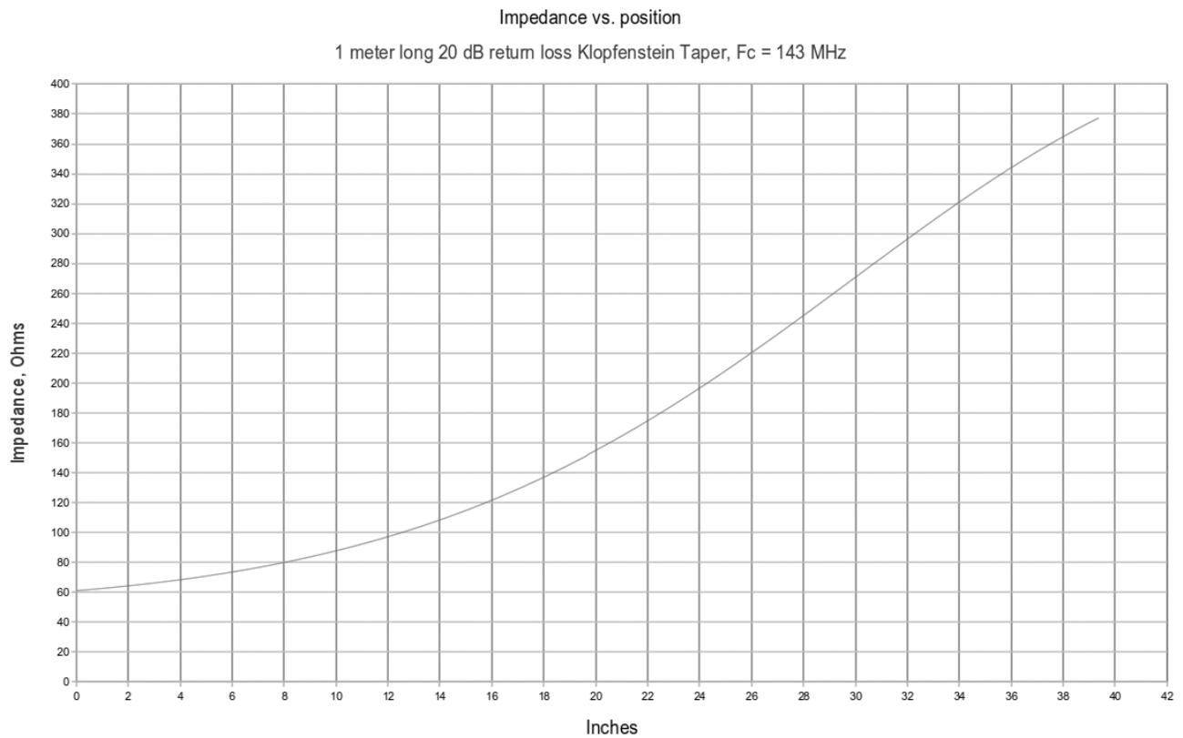
*Figure 6: Line Impedance vs. position for a 20 dB return loss Klopfenstein taper with corner frequency of 143 MHz.*
