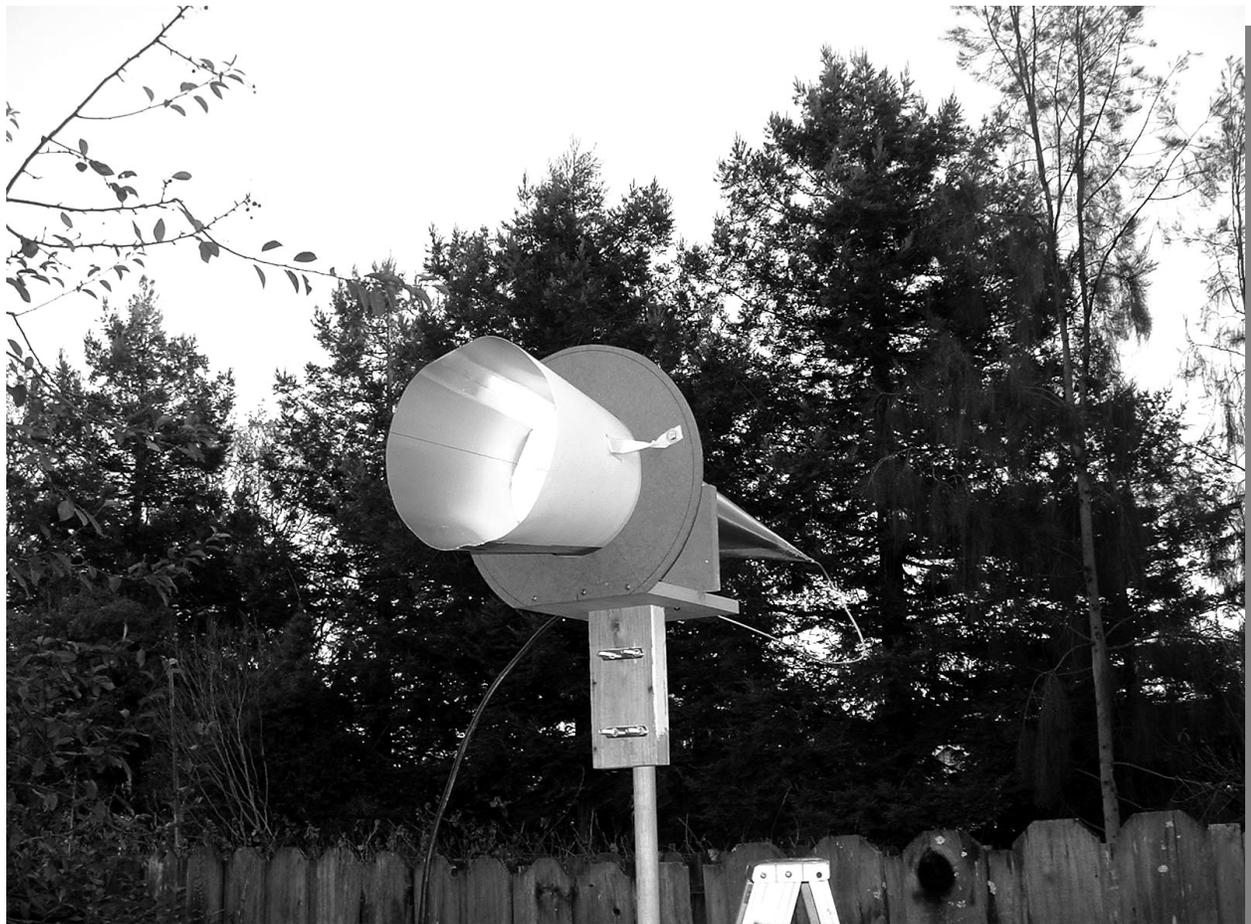
***Photo 1: Completed 144 MHz launcher mounted on a "holder". The #24 SWTL conductor extends from the center of the horn but is too small to be seen in this photograph.***
