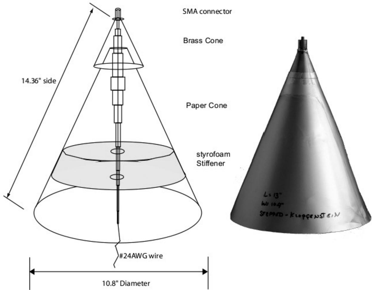
**Figure 3 Assembly of the 400 MHz Launcher**
