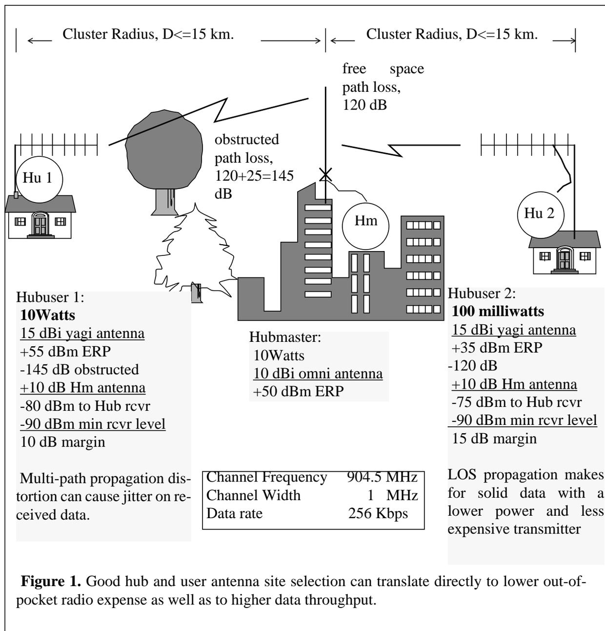
indicates the importance of careful selection of the Hubmaster site. While the hub doesn't have to be and shouldn't be high level, it should be LOS to each of the anticipated users. It is not necessary that the hub be at the physical center of a group of users. A very viable alternative is to locate it outside the cluster of users and use an antenna with directivity in both azimuth and elevation instead of the colinear with its omni-pancake pattern.
