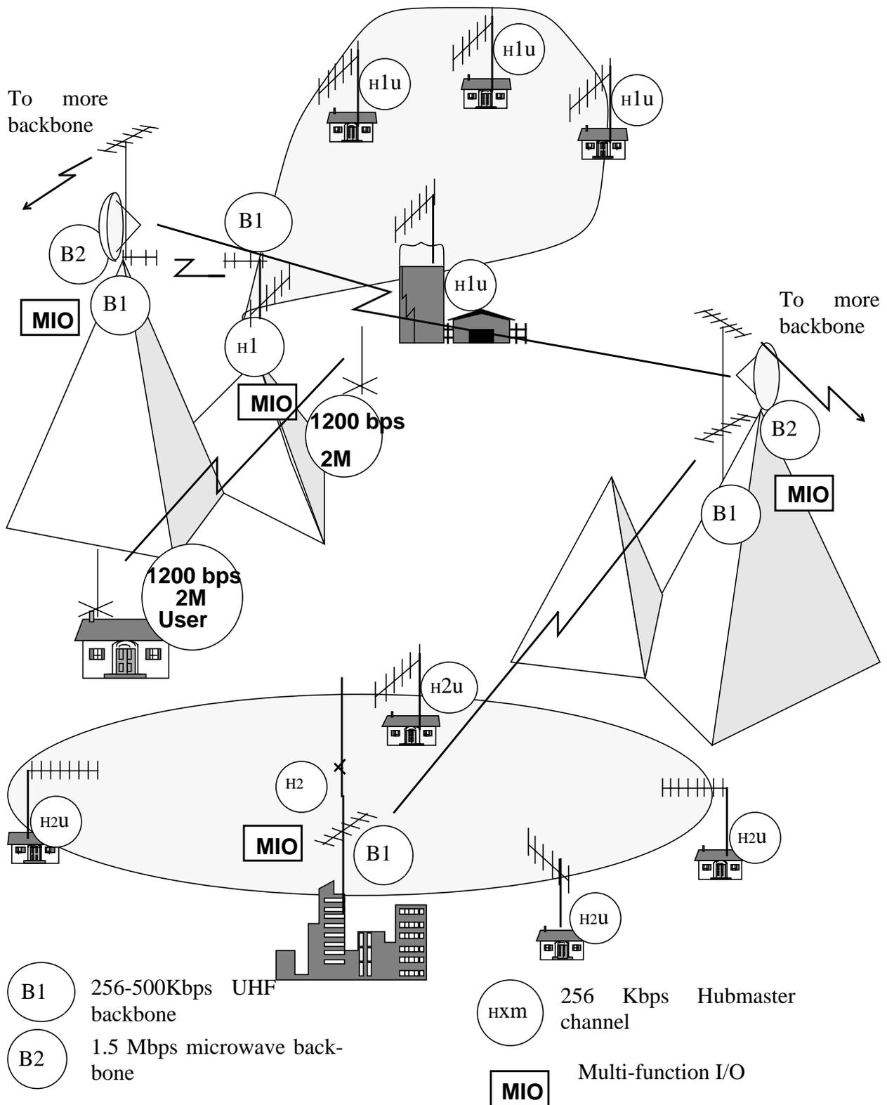
**Figure 2.** Common backbone and both high and low performance user access is provided in this example. LOS paths and directional antennas provide high performance with relatively inexpensive hardware.
