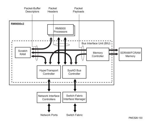
In Figure 3, both directions of data movement (switch inputs and switch outputs) are combined into single bidirectional paths. The example shows some of the methods by which specific parts of the data can be handled:
